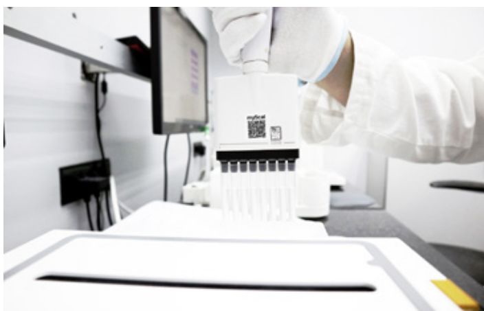
Picture 1. Using an 8-channel pipette in combination with Speedcal mobile and myScal® software solution reduce calibration time to 15 minutes.
