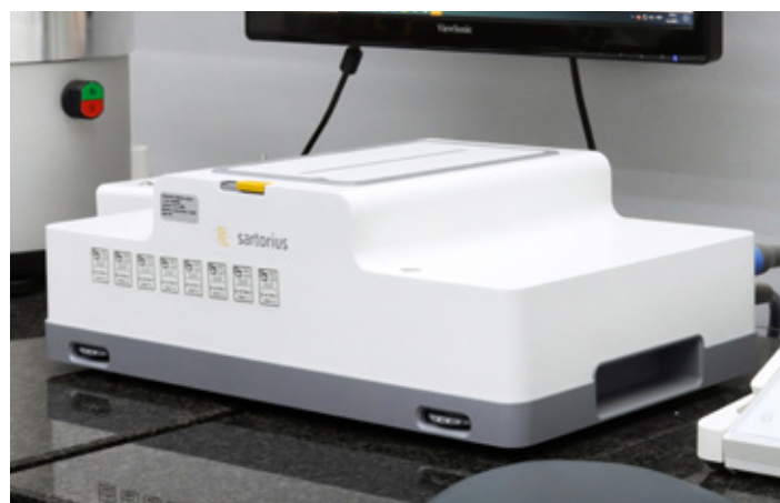
Picture 2. SpeedCal mobile is available with either 4, 8, or 12 channels, with the option of subsequently adding up to 12 channels.
